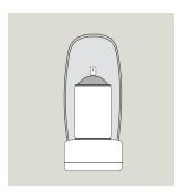
Open dispenser by pressing the button located on top of the unit. Remove the lid from the spray can and place inside the dispenser.
