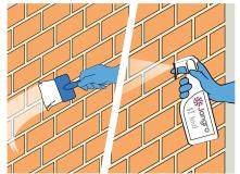
Apply to clean, dry walls. Paint or spray on, careful not to over apply (not too thick).
