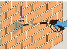
Pressure wash surface with hot water (>50°c).
